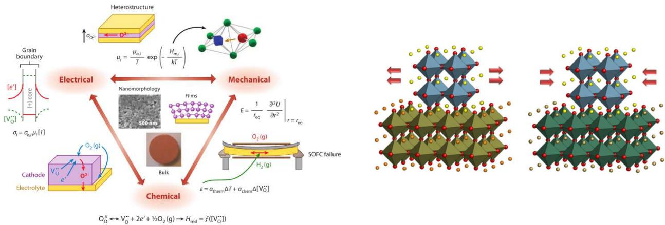
*Figure 1 a) Schematic representation of the electro-chemo-mechanical coupling (Tuller, 2011) b) Principle of inducing strain through substrate choice*
